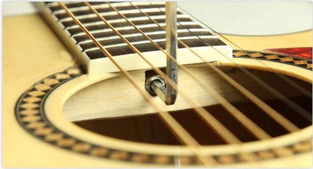
Diagram of the sound hole adjustment :
